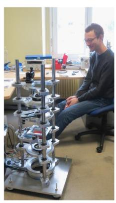
**Figure 2.** The automated optical bench—the heart slice embedded in MMA is positioned on a universal stage for the acquisition of the forty-nine images necessary to extract the orientation information.
