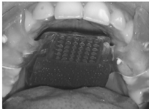
Fig. 1. Photograph of the wireless radio-controlled tongue-placed tactile output device used in the present experiment. It consists in a 2D electrodes array arranged in a 6 \times 6 matrix glued onto the inferior part of the orthodontic retainer which also includes microelectronics, antenna and battery.
