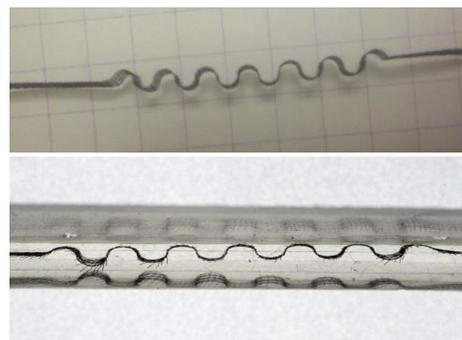
*Figure 2: Snake-like shaped NiTi textile, and down: composite with snake-like NiTi textile and silicone matrix*
