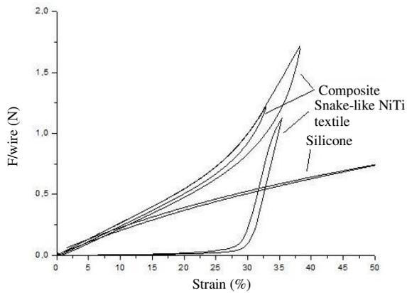
Figure 3: Tensile behavior of snake-like NiTi textile, silicone elastomer, and snake-like NiTi textile molded into silicone matrix
