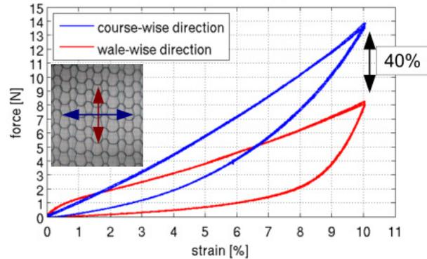
Figure 4: Mechanical behavior in tensile loading of knitted NiTi textile in course and wale direction [5]
