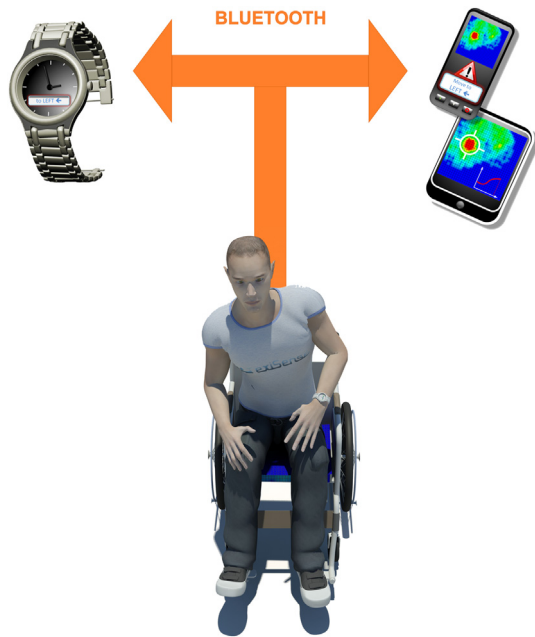
Figure 1 Principle of the TexiCare device: a dangerous situation triggers a wireless alert to the user by the mean of a watch or more sophisticated devices.
