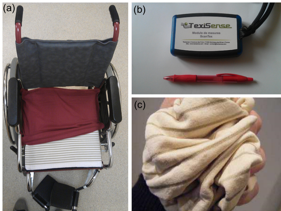
Figure 2 (a) TexiCare map around the cushion of a wheelchair; (b) The central unit connected to the map is approximately a cigarette box sized; (c) The TexiCare textile is thin, comfortable and washable.
