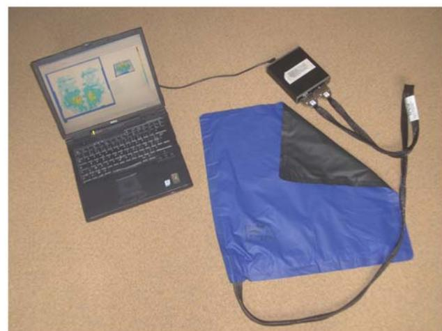
**Figure 2. Pressure map.** the VistaMedical Ltd. pressure mapping system connected to a laptop.
