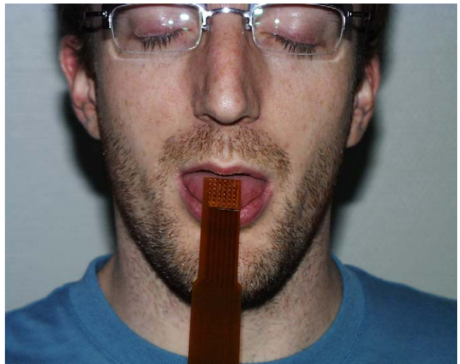
Fig. 1. Photograph of the Tongue Display Unit used in the present experiment. It comprises a 2D electrode array ( 1.5 \text{ cm} \times 1.5 \text{ cm} ) consisting of 36 gold-plated contacts each with a 1.4 mm diameter, arranged in a 6 \times 6 matrix.
