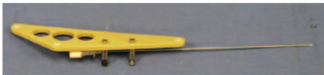
Figure 7 Needle equipped with a passive rigid body for position tracking.
