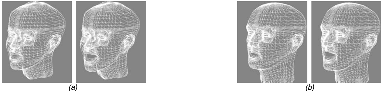
Figure 5: Building a generic talking face. Using an original 3D to 3D matching algorithm (Couteau, Payan et al. 2000), a generic “high definition” but static face mesh (see Figure 1.b) is scaled to multiple “low definition” motion capture data from each speaker. A “high definition” articulated clone for each speaker is then developed: (a) shows the neutral shape for two speakers (b) the shape deformation resulting from setting to +1 the “jaw opening” parameter.
