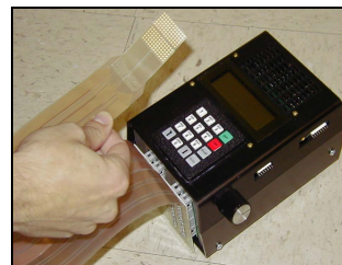
Fig. 1A. Wire TDU: 12 \times 12 matrix and flexible cable [2]
