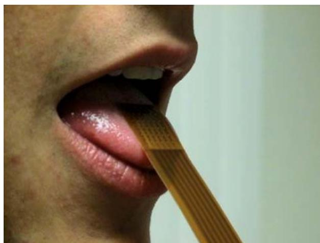
**Fig. 1** Photograph of the Tongue Display Unit used in the present experiment. It comprises a 2D electrode array ( $1.5 \times 1.5$  cm) consisting of 36 gold-plated contacts each with a 1.4 mm diameter, arranged in a  $6 \times 6$  matrix
