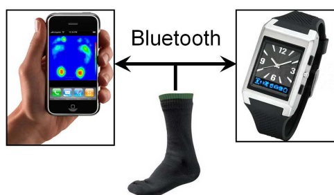
Fig. 1: Overview of the “smart sock” device.
