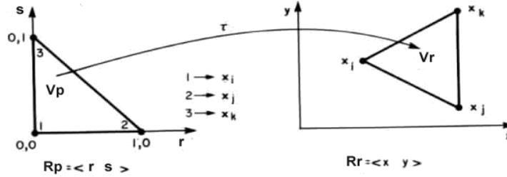
Fig. 1 : Transformation between the reference space, with a reference triangle, and the actual space, with an actual triangle. If this jacobian matrix of this transformation is not singular, FE analysis is allowed.
