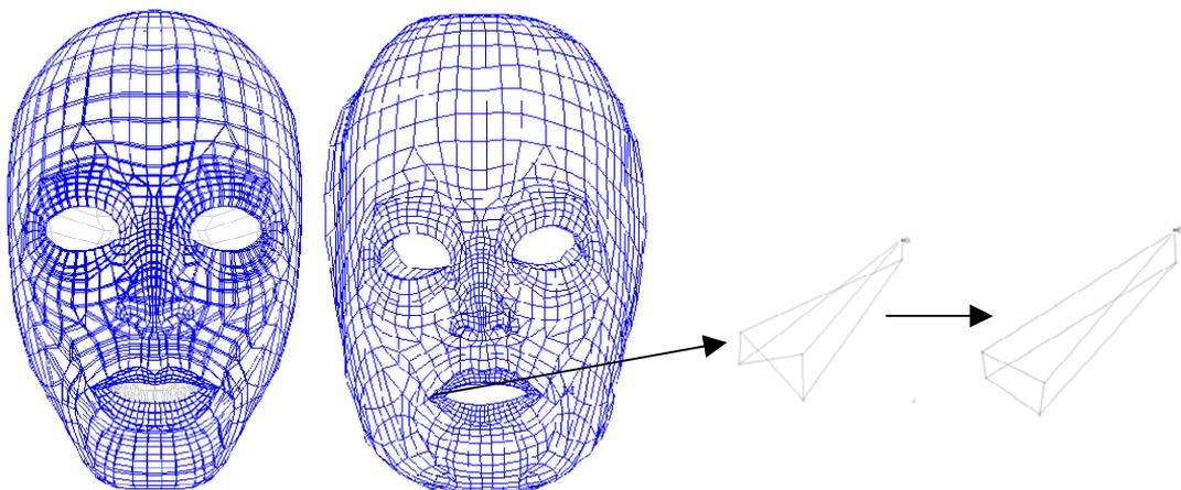
Fig. 4 : From left to right : the face FE atlas mesh; the patient FE mesh obtained with our method; an irregular element taken after the MM and regularized.
