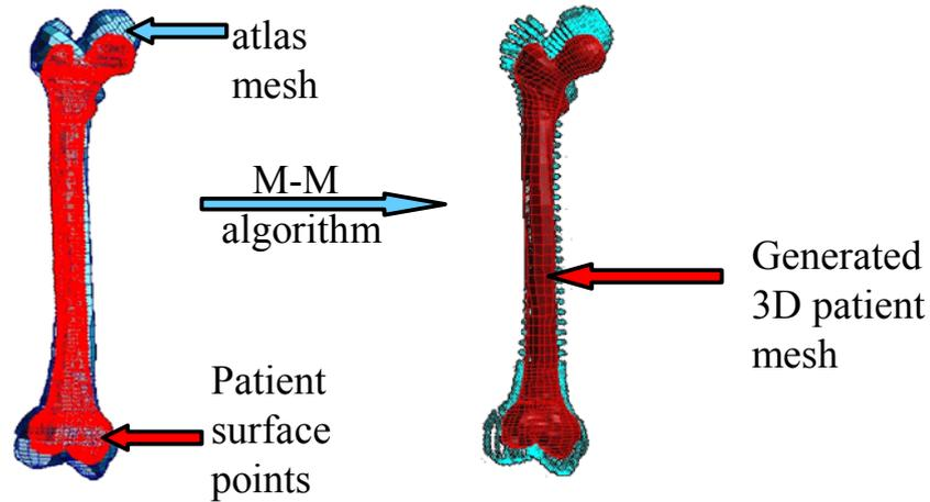
Fig. 3 : Application of the M-M algorithm to the femora FE mesh. The patient mesh is the smallest of the two meshes and is generated from the atlas mesh and the patient surface points.
