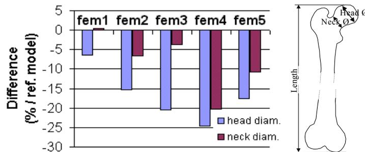
Fig. 2 : Difference of the head and neck diameter with respect to the reference model, on 5 FE meshes generated by the M-M algorithm
