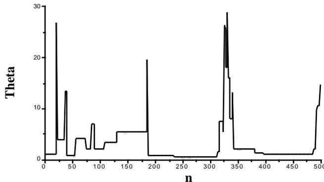
Notice that there are long flat periods (corresponding to all  $\theta^*$  values being rejected). Such a chain is called **poorly mixing**.
