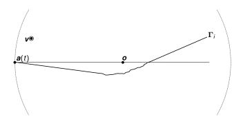
Cone-beam scanner with a circular source trajectory  $\mathbf{a}(t) \in \mathbb{R}^3$  around the axis defined by the isocenter  $\mathbf{o} \in \mathbb{R}^3$  and the unit axis  $\mathbf{v} \in \mathbb{R}^3$ .
