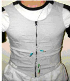
Figure 1. Computer-assisted RIP vest (Visuresp®, RBI, Meylan, France)
