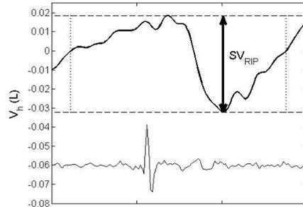
Figure 5. Extracted cardiac volume  $V_h$  and ECG signal for one cardiac cycle (defined by the dotted vertical lines). The stroke volume  $SV_{RIP}$  is estimated as the difference between the maximum and the minimum of the cardiogenic oscillation.
