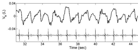
Figure 4. Cardiac signal  $V_h$  (bold line) extracted from the previous real  $V_{RIP}$  signal:  $V_h$  is the sum of IMFs 3 to 6, generated by CEEMD on  $V_{RIP}$  and considered as cardiac. ECG signal is shown to indicate each cardiac cycle.
