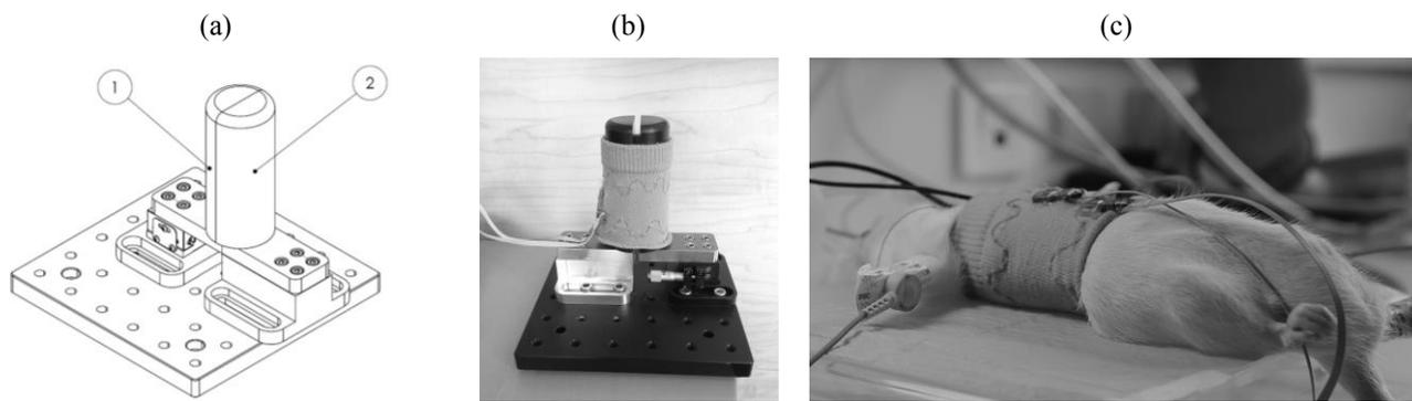
Figure 1. (a) Test bench. Volume surrounded by DECRO inductance plethysmography jacket is proportional to the distance separating the two half cylinders (1 and 2) that is controlled with a micrometric translation stage. (b) The DECRO inductance plethysmography jacket on the test bench. (c) Rat equipped with DECRO inductance plethysmography jacket device, mechanically ventilated and connected to ECG acquisition system.
