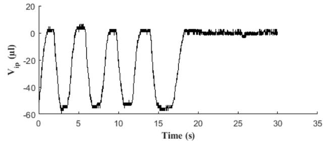
Figure 3. Experimental bench signal:  $V_{IP}$  volume recorded with DECRO IP jacket placed on the mechanical test-bench with repeated volume variations of 58  $\mu$ L. Last part of the signal (from 18 s) shows the noise level and quantization noise.
