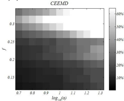
Fig. 7: Limits of agreement (in %) of Bland & Altman statistical tests between estimated  $SV_{CEEMD}$  and reference  $SV_{ref}$  for the 143 simulations.  $f$  is the frequency ratio ( $f_A/f_h$ ) and  $a$  is the amplitude ratio ( $a_A/a_h$ ).
