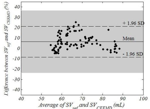
Fig. 5: Bland–Altman plot to compare the reference-based  $SV_{ref}$  with the CEEMD-based  $SV_{CEEMD}$  measurements of stroke volume (92 measures over 120 sec.). The gray domain represents the area of acceptance ( $\pm 30\%$ ).
