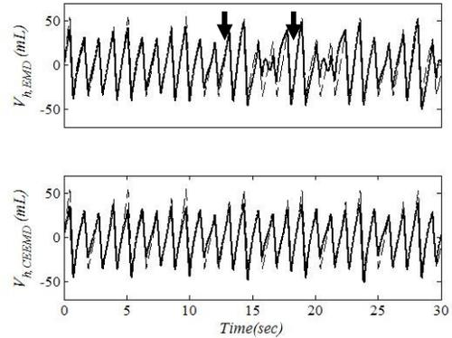
Fig. 4: Cardiac signals extracted (bold line) from the previous  $V_{th}$  signal:  $V_{h,EMD}$  is the  $IMF_{EMD}1$  on  $V_{th}$  and  $V_{h,CEEMD}$  is the sum of  $IMF_{CEEMD} 2$  to 5 on  $V_{th}$ . Simulated  $V_h$  signal (dashed line) is shown as reference.
