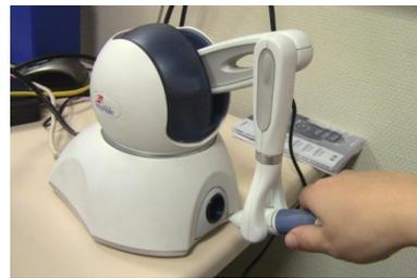
**Figure 4.** Omni Phantom device
