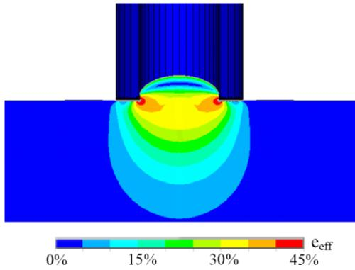
**Fig. 5.** Finite element calculation of the deformation under a 25 mbar negative pressure using the experimentally determined non linear constitutive law. The corresponding Von Mises strain values are provided.
