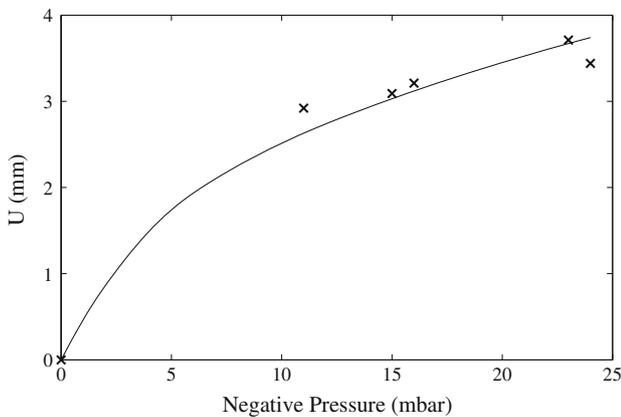
**Fig. 6.** Best fit of the experimental data (measured maximum height of the aspiration  $U$  vs. the applied negative pressure  $P$ ) and simulated data (non-linear Mooney–Rivlin constitutive law with  $a_{10} = 240$  Pa,  $a_{30} = 3420$  Pa and  $\nu = 0.45$ ).
